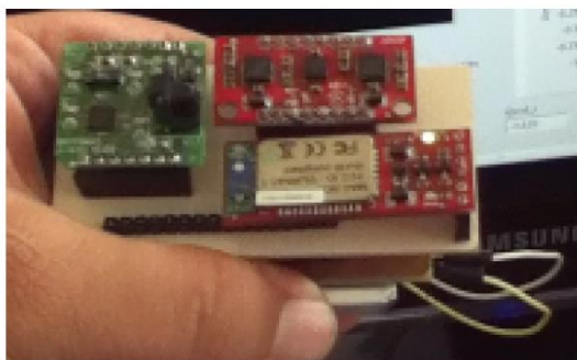
Figure 3. Implementation of AHRS prototype.
